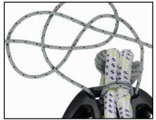
10. Further secure knot by carefully melting line ends with a hot knife.
