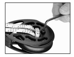
Secure loop to head of block with head securing line using a Carrick bend. For knot tying resources: www.harken.com/knots.
