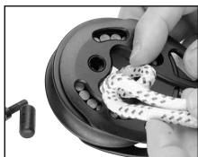
Pass loop ends through mouth so loops extend beyond block's sideplates as shown.
