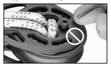
3. Inspect loops and lashings. Replace if there are signs of wear, or if the colored tracer fades from UV damage. Pull loop out of mouth and inspect loop/lashing carefully for any signs of wear, UV damage, fatigue, or strand separation. Replace loop if it shows signs of UV damage or wear.
